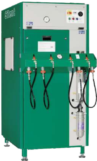
LW 160 E The user-friendly LW 160 E with electric drive is ideal for mobile applications or occasional filling operations
